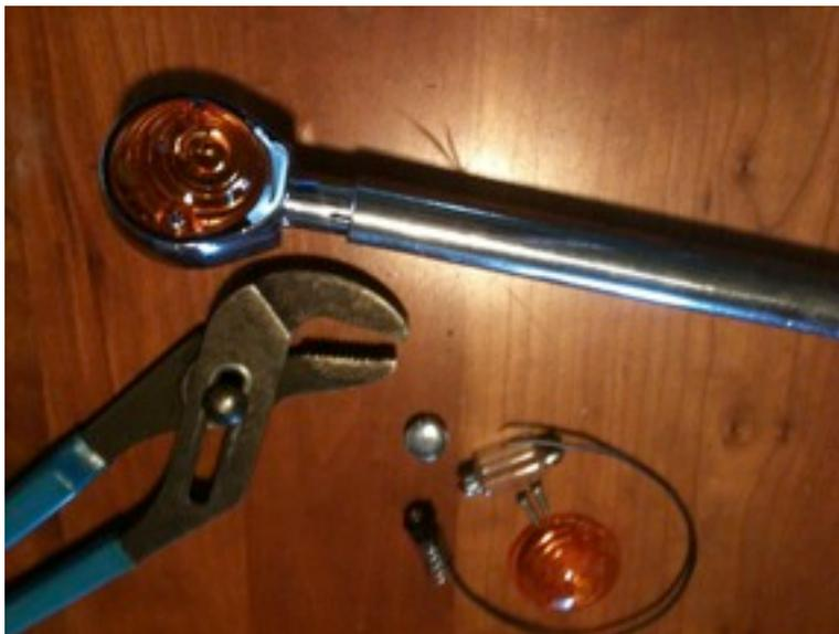
GENTLY compress the flanged end if necessary in order to get the narrow end to insert into your handlebar end. (Think inexpensive Taiwanese pot metal as you squeeze the pliers handles and say a little prayer to your mechanical gods of choice.)
