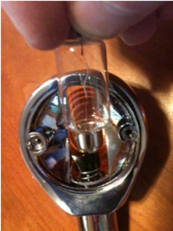
With the extra wire in place and the flange snugged up, just reinstall the bullet style bulb, re-attach the orange lenses and finally make the connection with the end cap screw. Now get a beer.. you deserve one.
